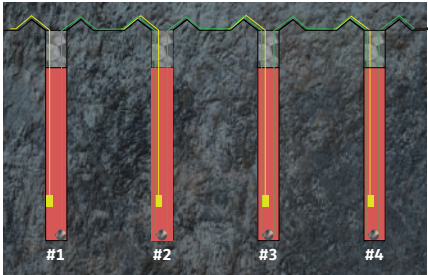
VOD TEST ON FOUR BLASTHOLES
