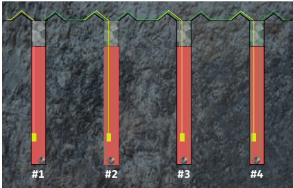
VOD TEST ON FOUR BLASTHOLES
