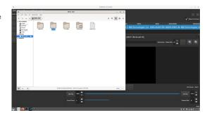
The video is recommended to have been saved to the SSD drive. In the image above, open the drive. In this drive, the video will be saved into the directory of DCIM if saving to TIF Stack. Inside this directory, there will be another directory called 100fastc shown to the right.
