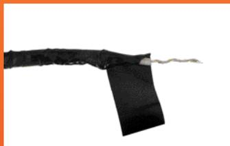
Making sure that there is no loose wires from the shielding touching the center conductors, continue to tape past the end.
