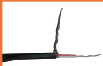
Twist the center conductors together.
