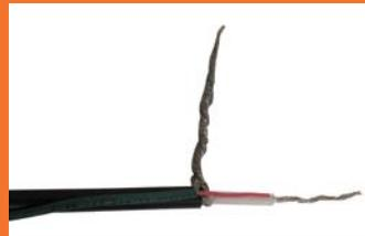
Twist the center conductors together.
