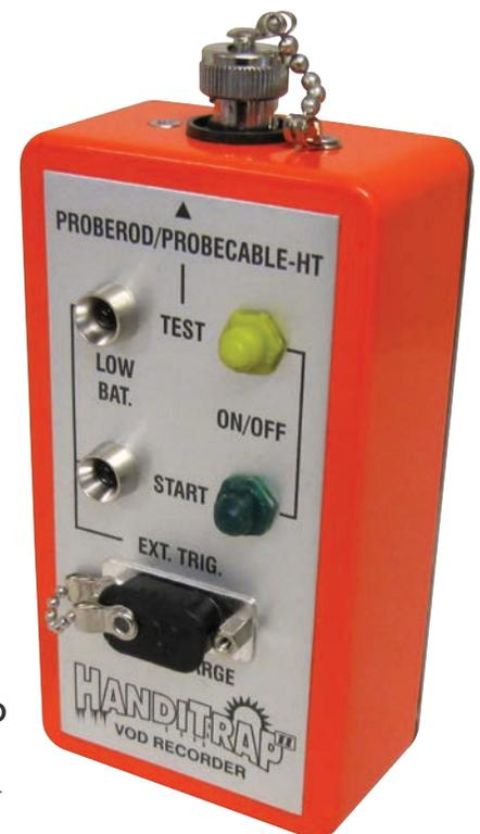
flashes quickly, the circuit exhibits a high resistance, or open circuit. Please refer to **Chapter 4.7** for possible solutions. Please note that the **START** button will be inactive so long as the resistance is not within the appropriate range. This fail-safe feature ensures that the User is notified of a faulty circuit before the test begins.
