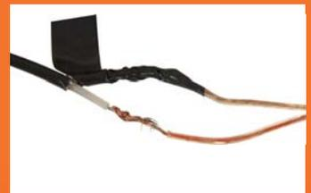
Place the RG-58/U Coaxial Cable beside the leads from the PROBECABLE-HT.
