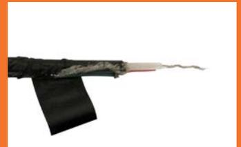
Pull the shielding wires back along the cables and start taping from the cable to the end.
