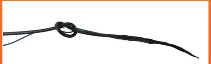
For strain relief, tie a loose knot down the cables from the connection as shown above.
