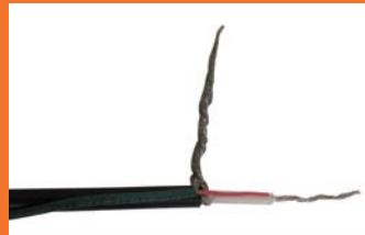
Twist the center conductors together.
