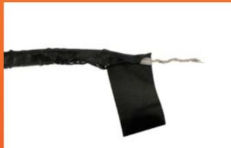
Making sure that there is now loose wires from the shielding touching the center conductors, continue to tape past the end.
