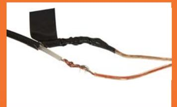
Place the RG-58/U Coaxial Cable beside the leads from the PROBEROD.
