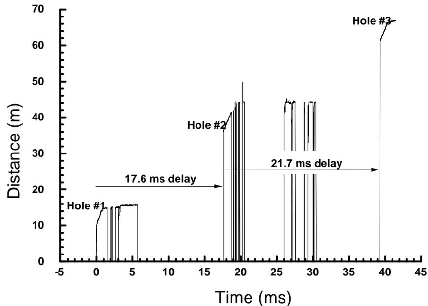
The operator can zoom in on each of the three holes to calculate the VODs in each hole and save the zoomed VOD results for each hole as sub-graphs as illustrated on the following page.
