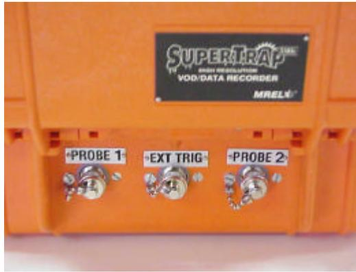
10. The probe setup aspects of the test are complete. The SuperTrap can now be set up to record the test.
