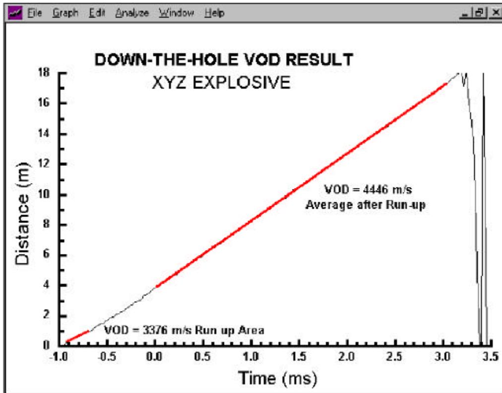
As detailed in **Section 3.3.2**, a typical VOD test on a multiple (3 in this case) blastholes using PROBEABLE is shown. Three 10 m deep holes were monitored. Each hole contained a column of approximately 5 m of explosives and the blast was tied in with a 17ms delay between holes.
