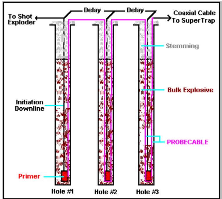
The data can be analyzed to determine the actual delays between holes and the VODs of the explosives in each of the holes.
