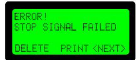
1. The continuity of the **Break Wire Sensor** was twisted around the sample and the detonation did not break the stop wire sensor.
