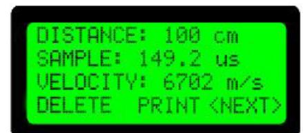
**Recorder** and review the screen. The screen should look similar to the image to the right. The velocity of the explosives will be shown in metres per second. Be sure to save the test by pressing the **Affirmative Check** button.
