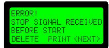
1. The sensor cables were reversed during the test.
