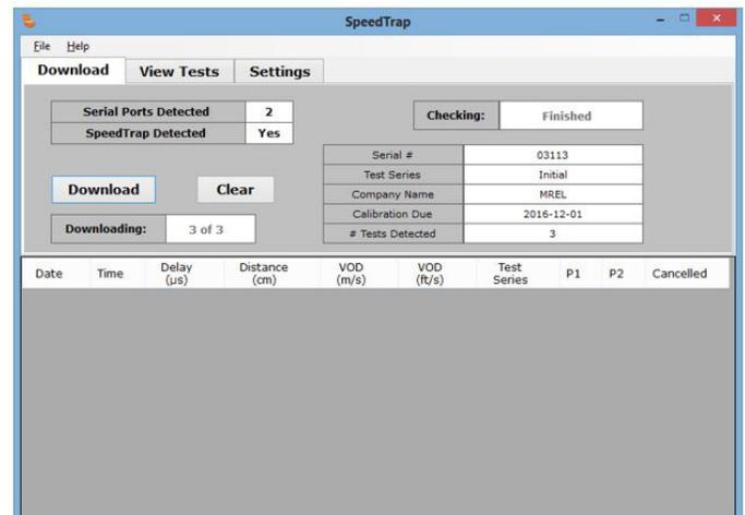
Please notice that below the **Download** button, the **Downloading** window shows the progression of the data streaming through the serial port. The two numbers will be equal when the downloading is complete.
