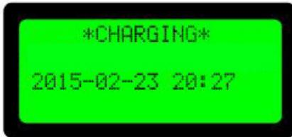
Once fully charged, the display will change to **\*CHARGED\***. The **SpeedTrap™ Velocity Recorder** is ready to be used.
