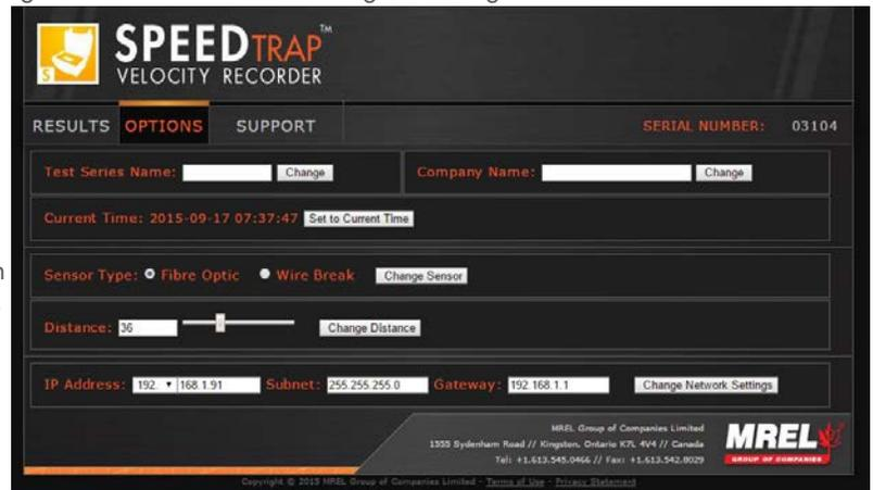
The **Adjustable Distance** (if purchased) can be changed between 5 and 100 cm in 1 cm increments and 1 and 10 m in 10 cm increments. There is two ways that the value can be changed. The slider can be moved until the desired value is shown in the box or the number can be directly typed in. The value can only be integers from 5 to 100 cm and single decimal from 1 to 10 m. The Change Distance button **MUST** be selected to confirm the change.
