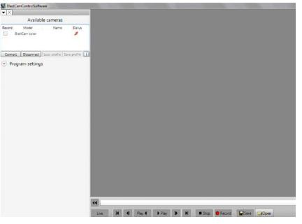
The found cameras will be listed in the "Available Cameras" section. Next, select the camera to use by clicking on the entry of this camera, then click on "**Connect**" to get the communication established with this camera. The camera's status symbol will change to green from red when the communication is established.
